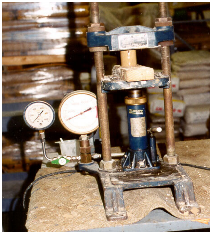
Fig. 3 – Compressive strength tests with Carver laboratory hydraulic unit
