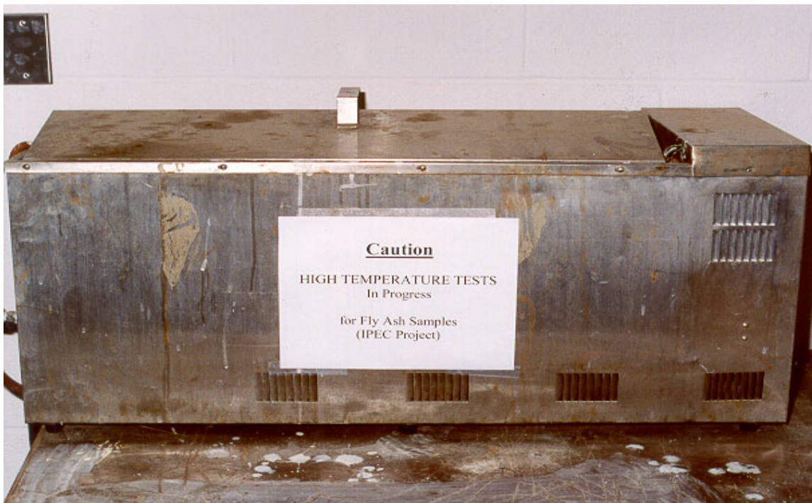
Fig 1 – Constant water temperature curing device
