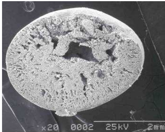
Figure 1. Scanning electron micrograph of cross section of a Bio-Sep® bead
