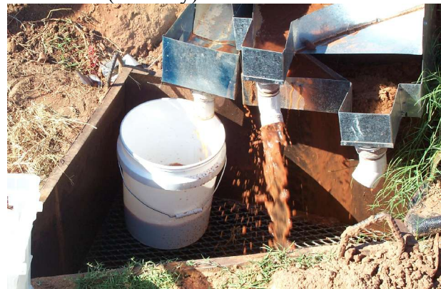
Figure 4. Sample collection troughs: left – through fence, center – through flow barriers, right – seepage under apron
