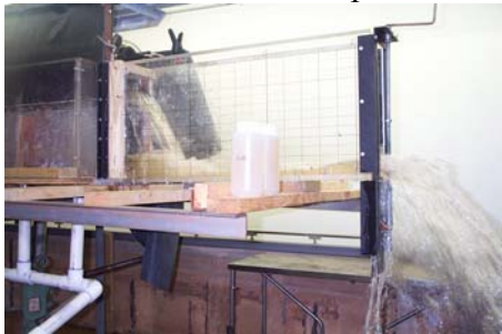
Figure 1. Laboratory flume to test erosion through apron
