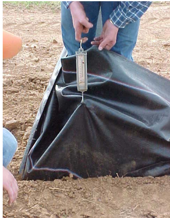
Figure 6. Test of anchoring in slot
