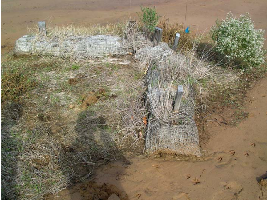
Figure 5. "V-shaped" fiber rolls and volunteer Baccharis on a roll & amendment plot at the Schuler Oil and Gas Field, south Arkansas, May 19, 2006.
