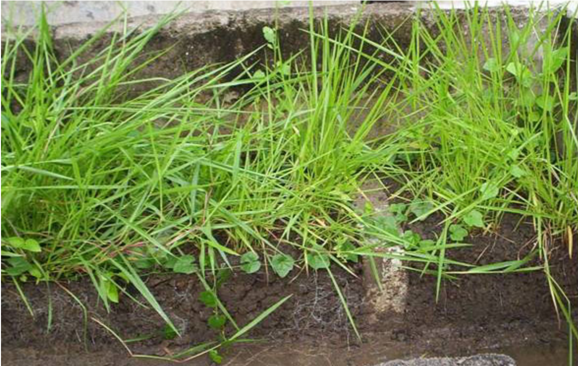
Figure 2. Growth of humidicola grass on sediments treated by chemical – biological stabilization.
