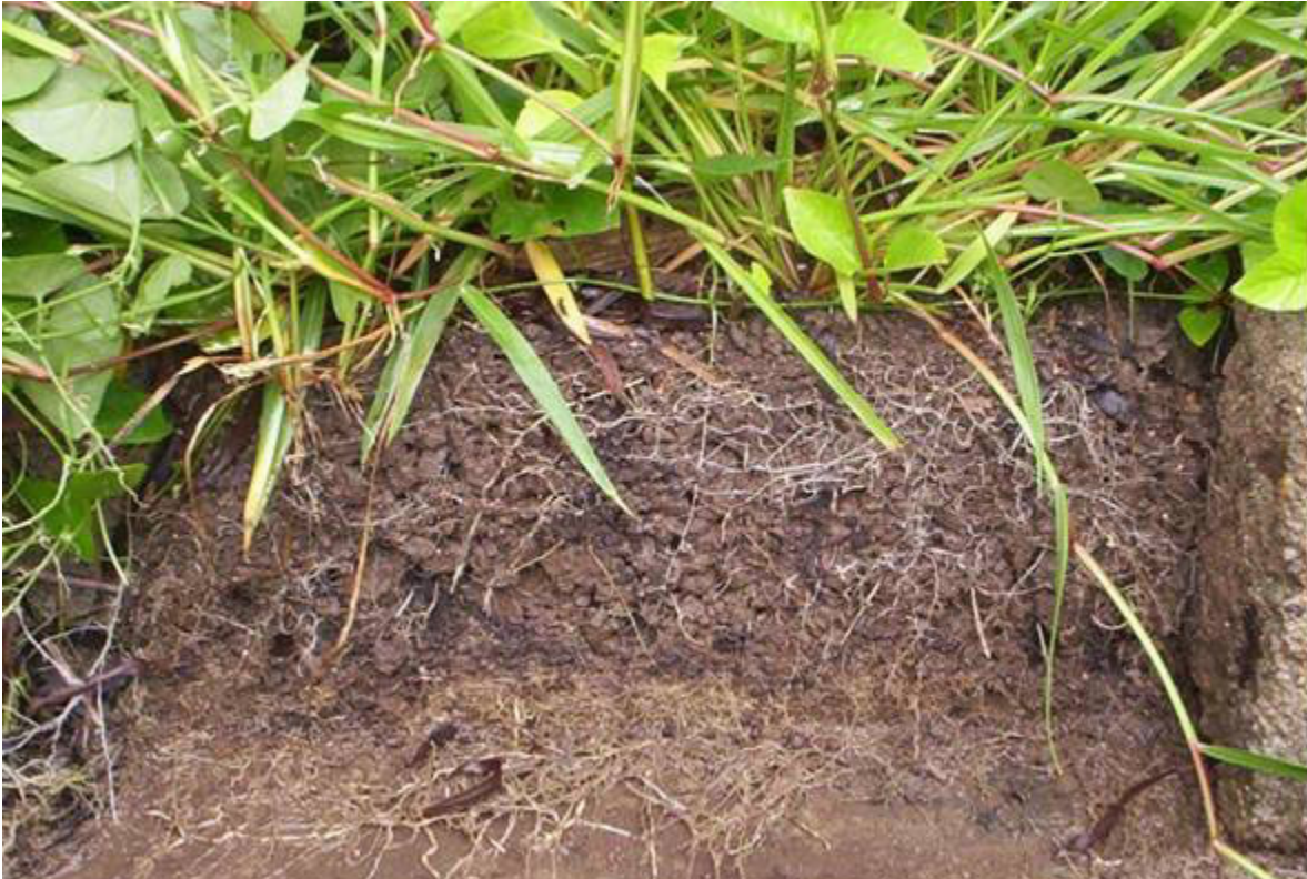
Figure 3. Root development ( Brachiaria humidicola ) in stabilized sediments.
