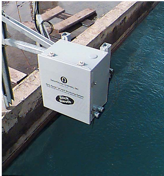
Figure 6. One of 5 units deployed at a Shell refinery (Australia) to monitor cooling water outfall channels. Photo courtesy Shell.
