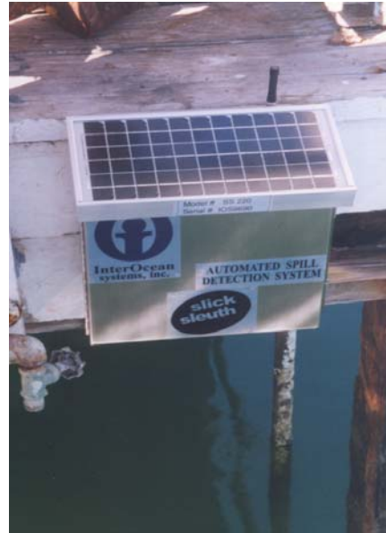
Figure 4. Early production unit. DC/Solar power, radio telemetry.
