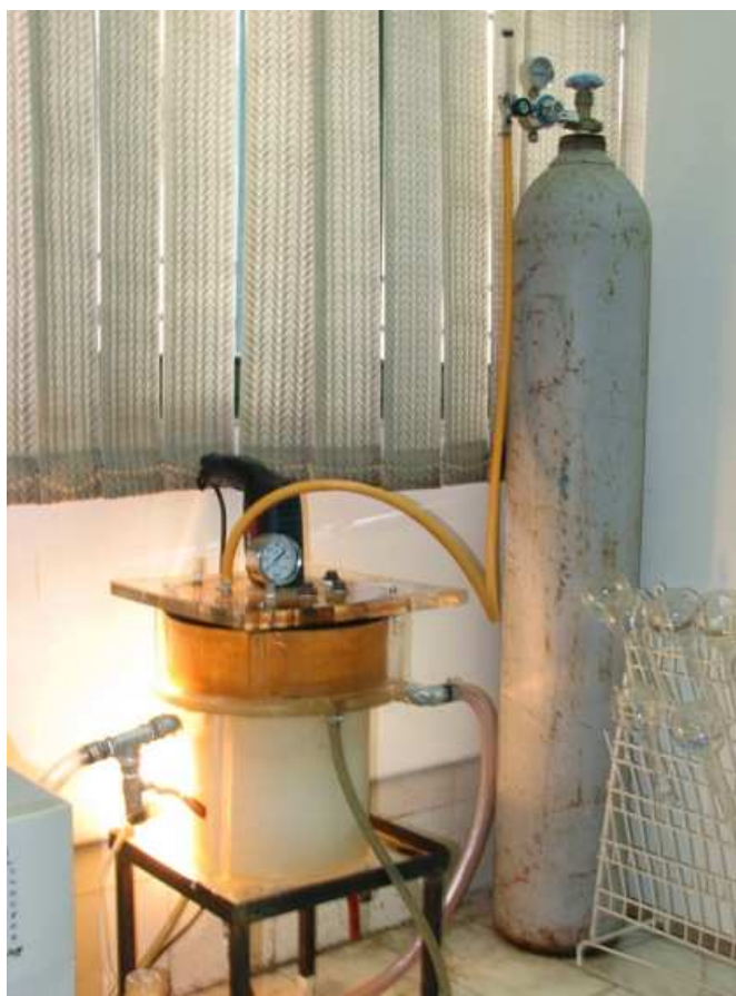
Figure 1. IGF pilot set up: IGF flotation cell and the nitrogen capsule Feed Gas
