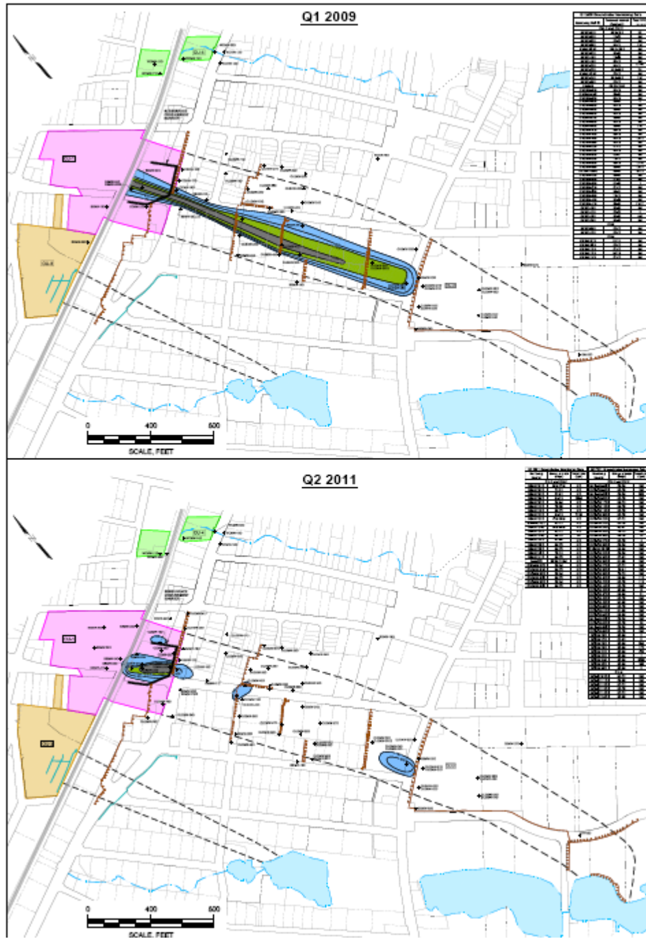
Figure 13 – Total PAH Deep Zone Isoconcentration Lines
