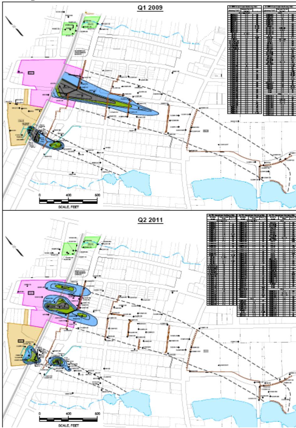
Figure 8 – Total BTEX Shallow Zone Isoconcentration Lines
