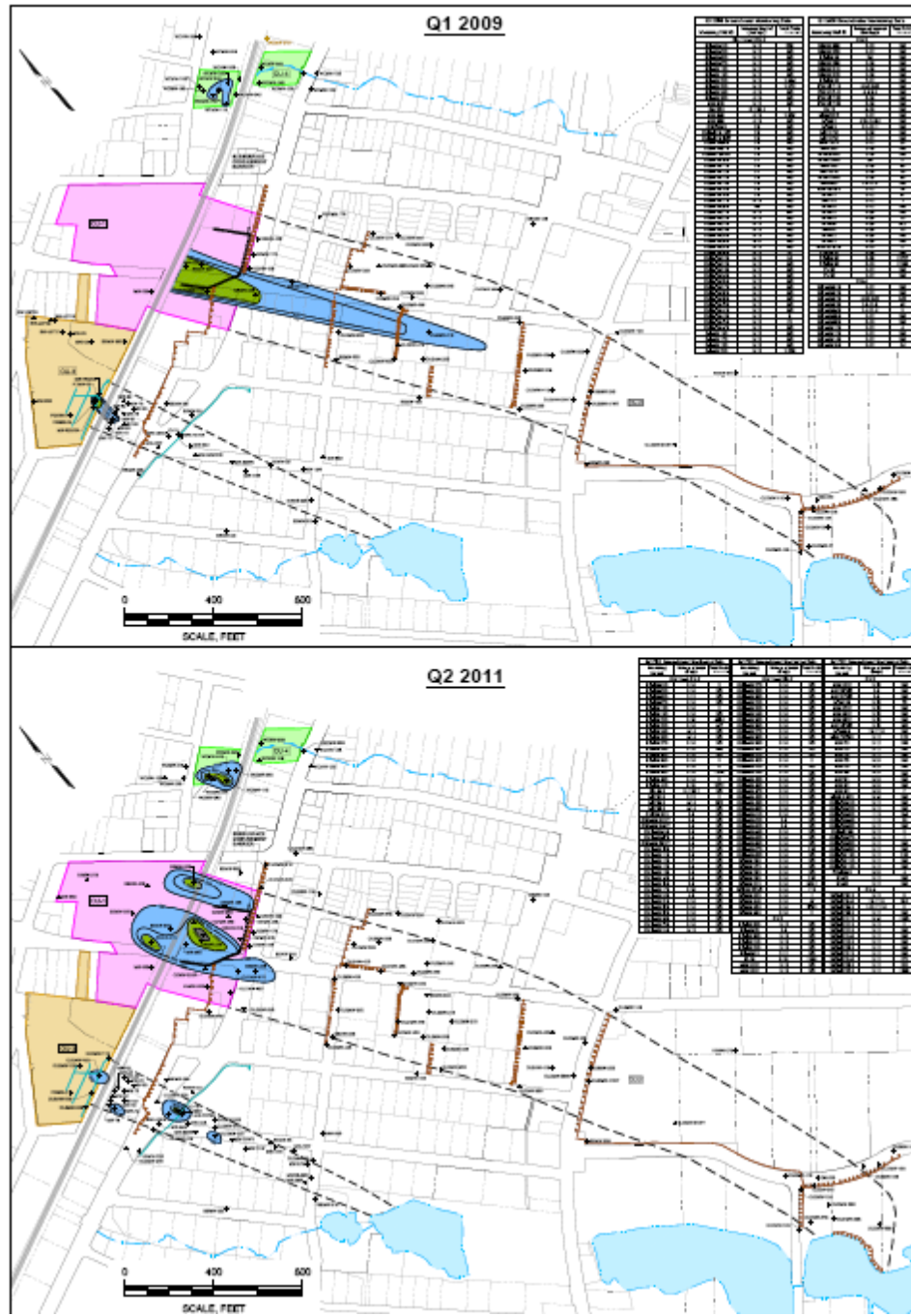
Figure 9 – Total BTEX Intermediate Zone Isoconcentration Lines
